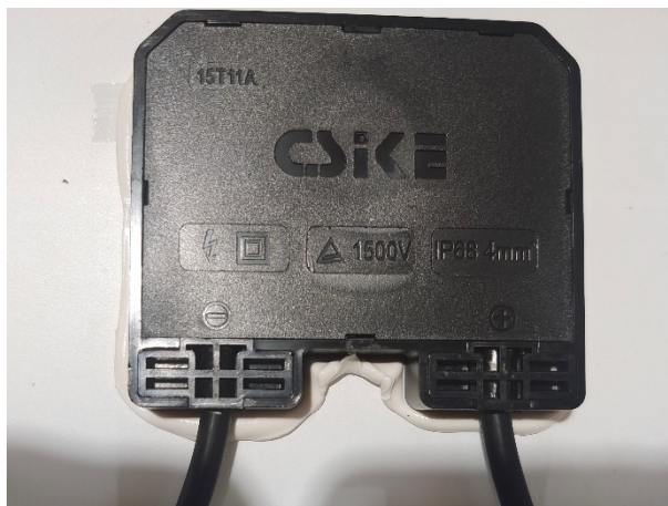
Fig. 3: View of junction box of module type ESPMC335
